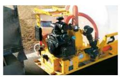
**MODULAR DESIGN.** Allows the power pack to be mounted on either end of the tank or trailer, enhancing operator accessibility to the unit.
